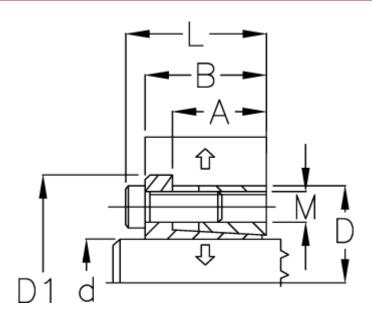
A mm = 25 B mm = 33 D1 mm = 88 d H8 mm = 30 D mm = 80 F kN torque = 72 L mm = 41 M mm = M8 P N/mm2 surface pressure on shaft/hub = 108T N m torque = 1077Ts N m bolt tightening torque = 41
